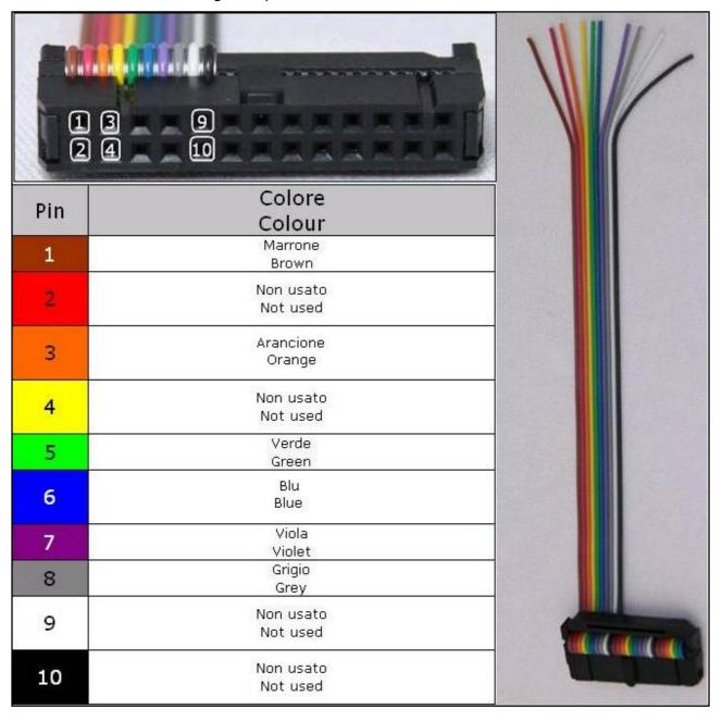
Connect the BOOT GREY wire of the F32GN037C cable as shown here below:
