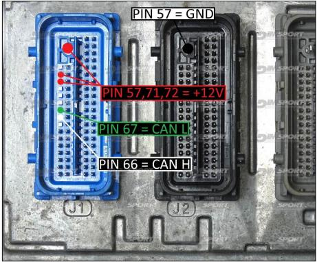
To the power feeding pins 57, 71, 72 (+12V) you can connect both wires red (VECU) and orange VKEY) of the F32GN037C/D cable, they both have 12V signal.
