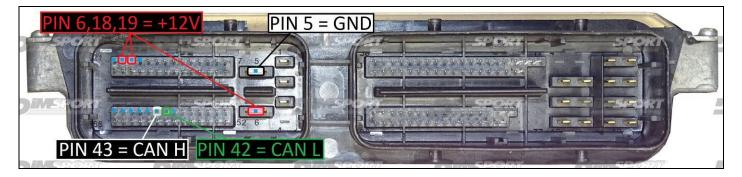
To the power feeding pins 6,18,19 (+12V) you can connect both wires red (VECU) and orange VKEY) of the F32GN037C/D cable, they both have 12V signal
