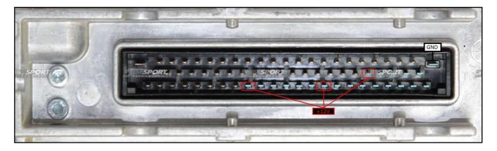
To power the ECU it is possible to use the VKEY wirings too, both red and orange wires are 12V.
