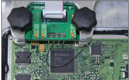
A different solution is to connect the BOOT wire directly to the orange BOOT clamp on the DIMA adapter F34DM011. Check that the yellow BOOT jumper is set in ON position. Connect the DIMA flat cable to the Trasdata.
