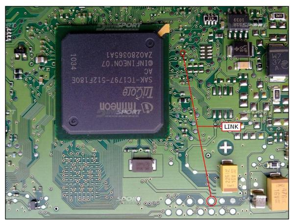
A different solution is to connect the BOOT wire directly to the orange BOOT clamp on the DIMA adapter F34DM011. Check that the yellow BOOT jumper is set in ON position. Connect the DIMA flat cable to the Trasdata.
