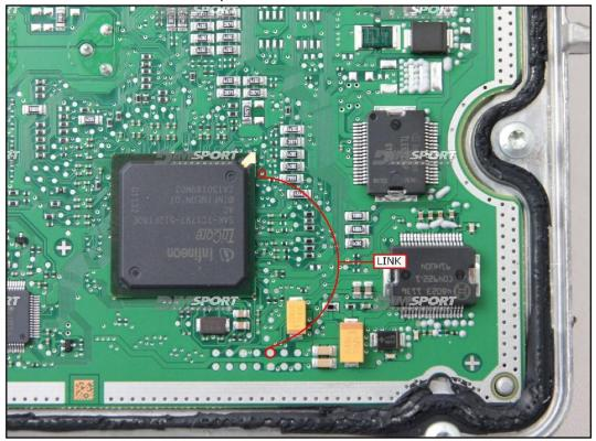
A different solution is to connect the BOOT wire directly to the orange BOOT clamp on the F34DM011 adapter. Check that the yellow BOOT jumper is set in ON position. Connect then the flat cable to the Trasdata.
