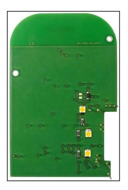
Here below the communication pads for the F34DM026 adapter are displayed.
