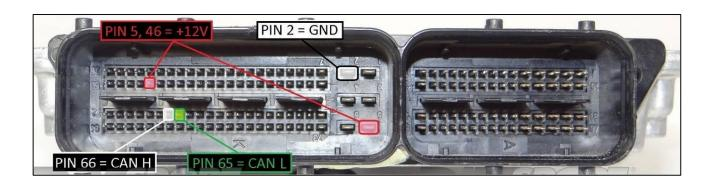
Attention: for a correct communication it is necessary to create a short circuit between the CAN pins of the microprocessor. The two short circuits **LINK 1 & LINK 2** (yellow link in the following picture) needs two in line resistors of 470 ohm (one resistor each bridge). Remove these bridges and resistors before setting the ECU back into the vehicle.
