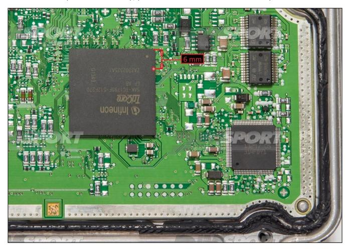
For a safe procedure the Trasdata flat cable must be disconnected from the DIGITAL PORT. The ball to clamp is the 6th one from the right corner of the micro
