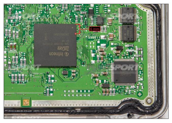
You need to clamp the sixth ball only, please check here below how to identify it. Connect the clamp to the ball first, then the clamp to the F34DM011 adapter and ONLY AFTER connect the F34DM011 adapter to the Trasdata.
