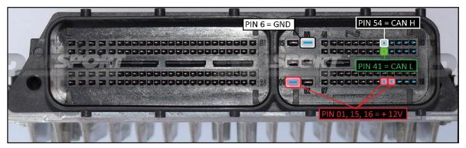
To the power feeding pins 01,15,16 (+12V) you can connect both wires red (VECU) and orange VKEY) of the F32GN037C cable, they both have 12V signal.
