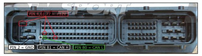
To the power feeding pins 4,61,77 (+12V) you can connect both wires red (VECU) and orange (VKEY) of the F32GN037C cable, they both have 12V signal.
