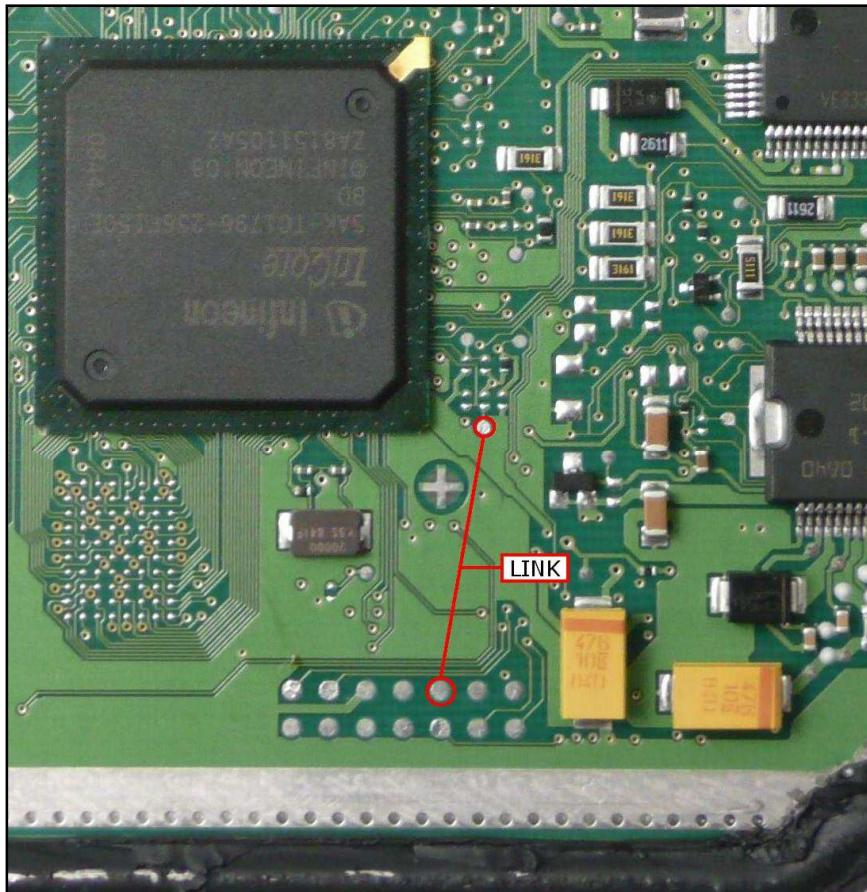
A different solution is to connect the BOOT wire directly to the orange BOOT clamp on the DIMA adapter F34DM011. Check that the yellow BOOT jumper is set in ON position.
