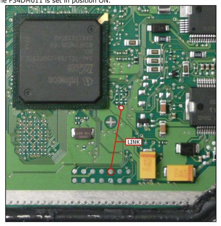
A different solution is to connect the BOOT wire directly to the orange BOOT clamp on the DIMA adapter F34DM011. Check that the yellow BOOT jumper is set in ON position. Connect the DIMA flat cable to the Trasdata.
