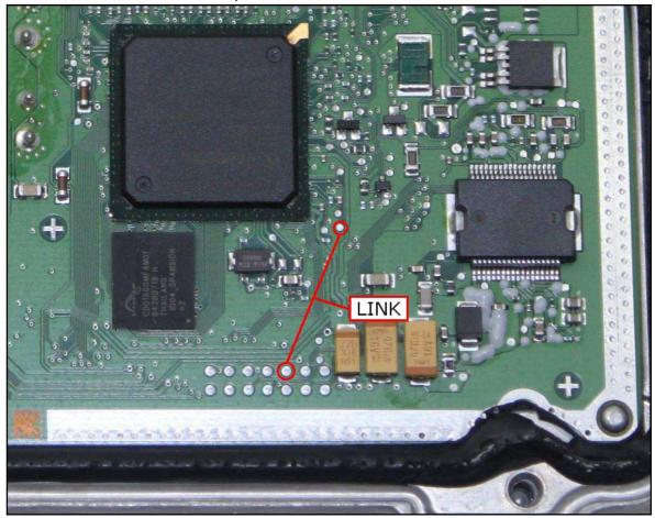
A different solution is to connect the BOOT wire directly to the orange BOOT clamp on the DIMA adapter F34DM011. Check that the yellow BOOT jumper is set in ON position. Connect the DIMA flat cable to the Trasdata.
