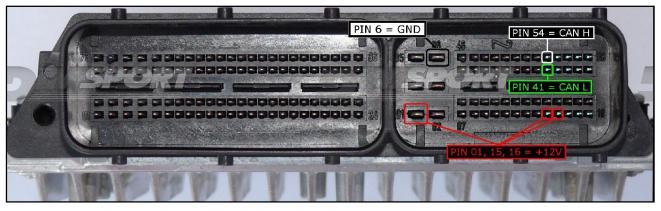
WARNING: to the power feeding pins 01,15,16 (+12V) you can connect both wires red (VECU) and orange VKEY) of the F32GN037C cable, they both have 12V signal.
