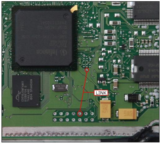
A different solution is to connect the BOOT wire directly to the orange BOOT clamp on the DIMA adapter F34DM011. Check that the yellow BOOT jumper is set in ON position. Connect the DIMA flat cable to the Trasdata.
