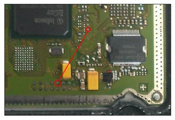
A different solution is to connect the BOOT wire directly to the orange BOOT clamp on the DIMA adapter F34DM011. Check that the yellow BOOT switch is set in ON position. Connect the DIMA flat cable to the Trasdata.
