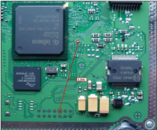
A different solution is to connect the BOOT wire directly to the orange BOOT clamp on the DIMA adapter F34DM011. Check that the yellow BOOT jumper is set in ON position. Connect the DIMA flat cable to the Trasdata.
