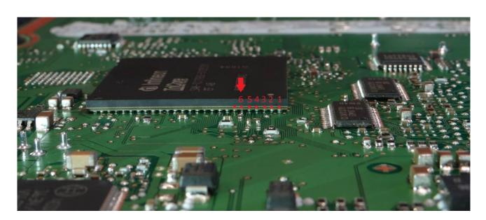
Connect the GREY wire of the F32GN037C cable to the micro clamp and the the micro clamp to the sixth ball of the Micro.
