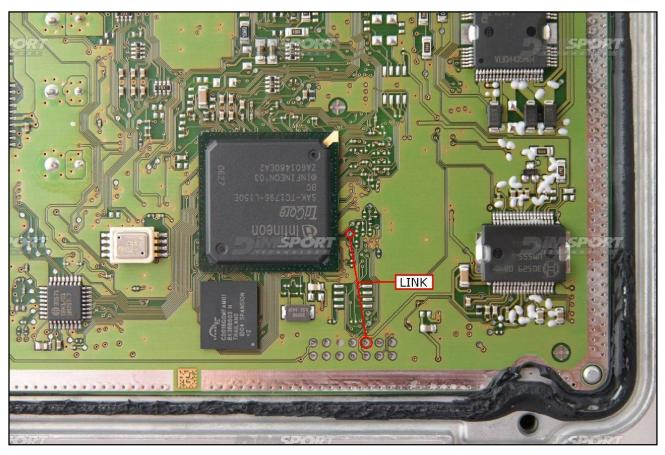
A different solution is to connect the BOOT wire directly to the orange BOOT clamp on the F34DM011 adapter. Check that the yellow BOOT jumper is set in ON position. Connect the DIMA flat cable to the Trasdata.
