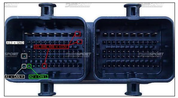
To connect to the pin 5,48,56 it is possible to use the red and orange wires, they both are 12V.
