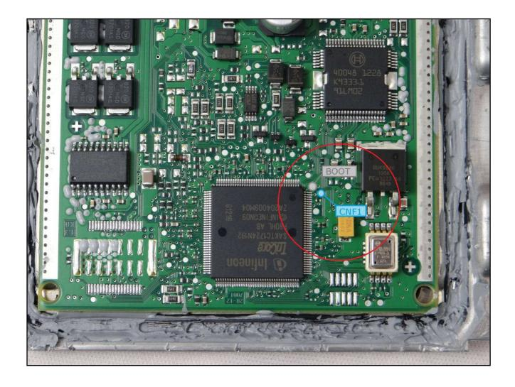
**BOOT/CNF1 CONNECTION for TURBO engine**Connect the GREY and BLUE wires of the cable F32GN037C as described here below:
