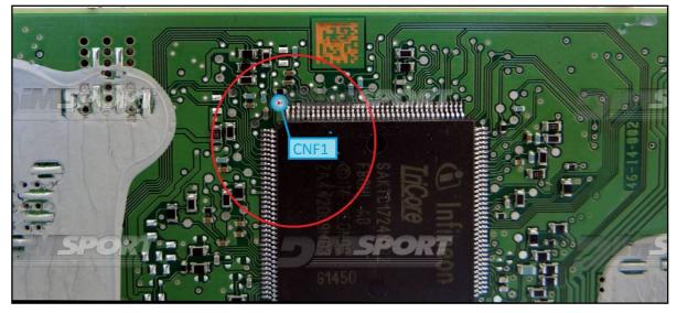
The BOOT pad is placed on the board side without the MPC.
