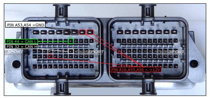
To the power feeding pins A16,A55,A56 (+12V) you can connect both wires red (VECU) and orange VKEY) of the F32GN037C/D cable, they both have 12V signal.
