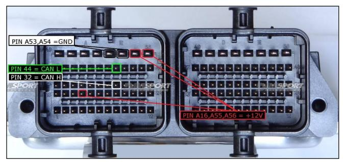
It is possible to use RED and ORANGE wirings for the pins A16,A55,A56, they all are +12V signals.
