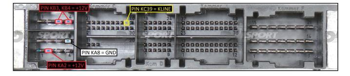
To the pin KB3,KB4,KA2 you can connect both wires red and orange, they both have 12 Volt signal.
