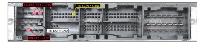
To the power feeding pins KB3,KB4,KA2 (+12V) you can connect both wires red (VECU) and orange VKEY) of the F32GN037C cable, they both have 12V signal.
