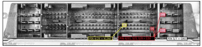
To the 12V power feeding pins you can connect both wires red and orange, they both have 12 Volt signal.
