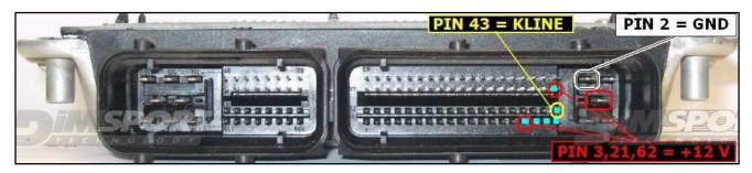
To the pin 3,21,62 you can connect both wires red and orange, they both have 12 Volt signal.
