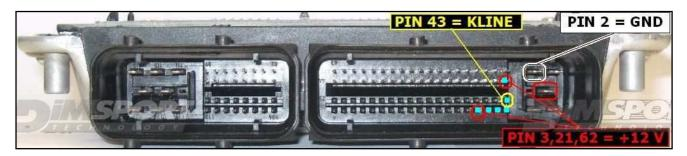
To the pin 3,21,62 you can connect both wires red and orange, they both have 12 Volt signal.
