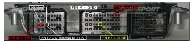
Warning: for a correct ECU power feeding it is necessary to connect a 10Kohm resistor between the PIN F2 and the PIN G2 +12V.
