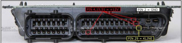
To the pin 4,15,51 you can connect both wires red and orange, they both have 12 Volt signal. **BOOT&CNF1 CONNECTION**
