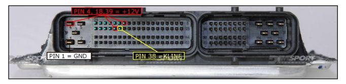
To the pin 4,18,39 you can connect both wires red and orange, they both have 12 Volt signal.
