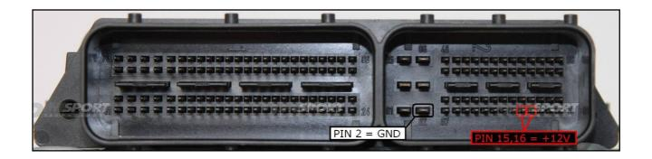
**F34NTA06 adapter connection**The triangle symbol on the adapter board must not be considered a valid reference.
