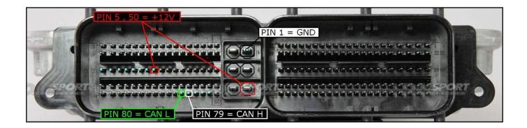
**BOOT/POL4 CONNECTION**Connect the GREY wire of the cable F32GN037C/D as described here below :
