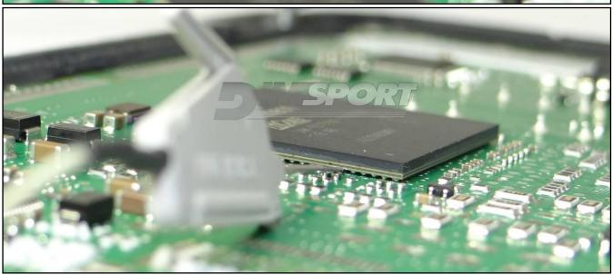
Connect the clamp wire directly to the BOOT clamp on the DIMA F34DM011 adapter. Check that the yellow BOOT jumper is set in ON position. Connect the DIMA flat cable to the Trasdata.
