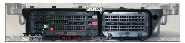
**BOOT/POL4 DIRECT CONNECTION**Connect the GREY wire of the cable F32GN037C as described here below:
