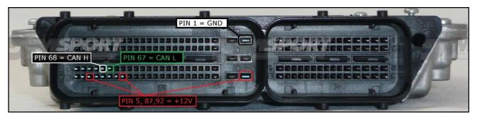
To the power feeding pins 5, 87, 92 you can connect both wires red and orange, they both have 12 Volt signal.
