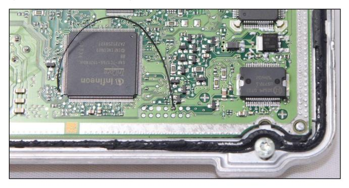
A different solution is to connect the BOOT wire directly to the orange BOOT clamp on the DIMA adapter F34DM011. Check that the yellow BOOT jumper is set in ON position. Connect the DIMA flat cable to the Trasdata.
