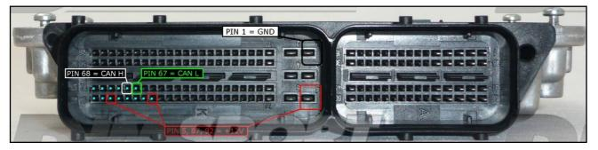
To the 3 power feeding pins 5,87,92 you can connect both wires red and orange, they both have 12 Volt signal.
