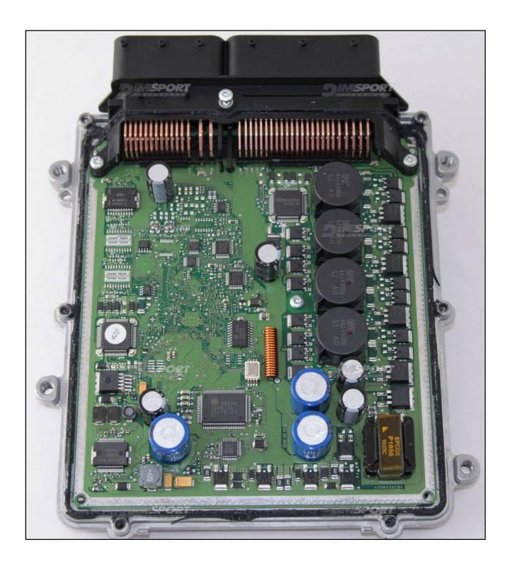
On this ECU POL4/BOOT pin is located on the lower side of the board, therefore you must detach the lower cover of the ECU too. This operation must be performed very carefully. After detaching the board from both covers reassemble them on the board, tighten the screws back to the covers and test the ECU on the vehicle. Start the vehicle.
