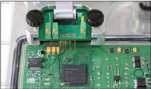
A different solution is to connect the BOOT wire directly to the orange BOOT clamp on the adapter. Check that the yellow BOOT jumper is set in ON position. Connect the flat cable to the Trasdata.
