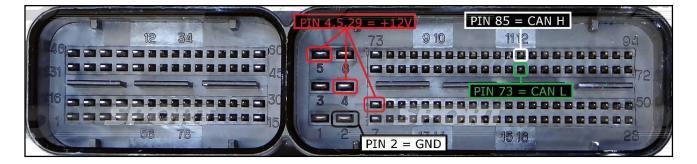
To connect to the pin 4,5,29 it is possible to use the red and orange wires, they both are 12V.
