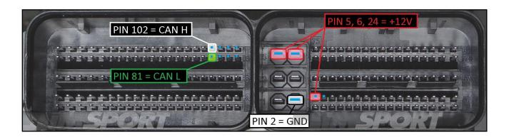
To the power feeding pins 5,6,24 (+12V) you can connect both wires red (VECU) and orange VKEY) of the F32GN037C cable, they both have 12V signal.
