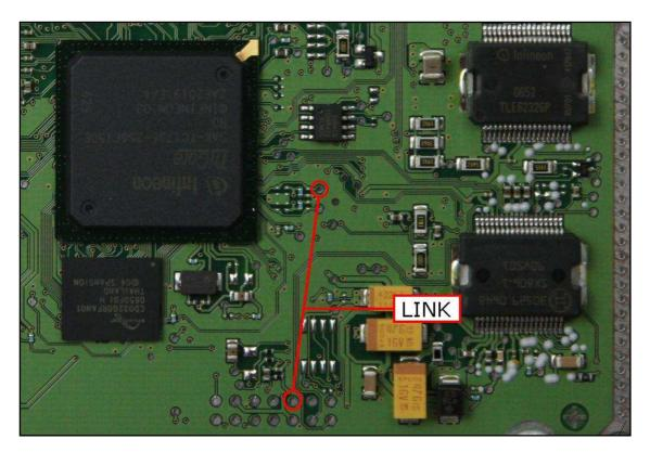
A different solution is to connect the BOOT wire directly to the orange BOOT clamp on the DIMA adapter F34DM011. Check that the yellow BOOT jumper is set in ON position. Connect the DIMA flat cable to the Trasdata.
