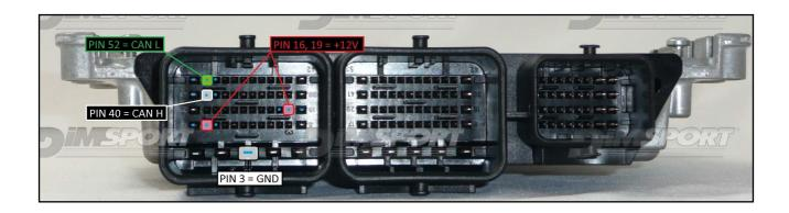
**BOOT/POL4 CONNECTION - MED172(TURBO)**Connect the GREY wire of the cable F32GN037C as described here below:
