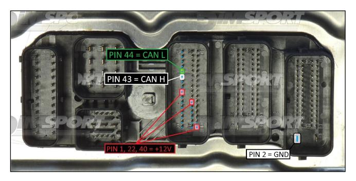
To the power feeding pins 1,22,40 (+12V) you can connect both wires red (VECU) and orange (VKEY) of the F32GN037C cable, they both have 12V signal.
