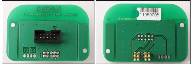
**WARNING** : in order to write the ECU it is necessary to create the little bridge LINK that enables the writing process on the EXTERNAL FLASH. Remove it at the end of the writing process.
