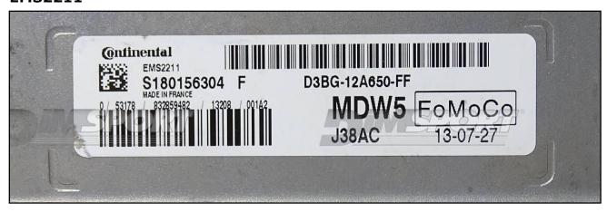
WARNING: for these ECUs it <u>could be</u> necessary to perform the PWD recovery via ObdData by connecting the Trasdata to the vehicle OBDII socket.
