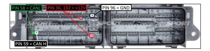
For a correct communication with the ECU it is necessary to connect a 100 Ohm resistor as displayed in the following picture, on the microprocessor ECU side. Remove the resistor before placing the ECU back into the vehicle.
