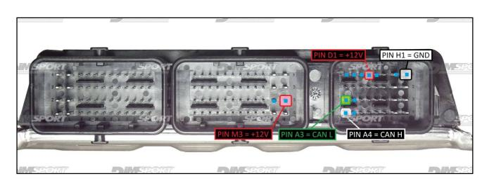
WARNING: due to the relevant power absorbed by the ECU at the beginning of the communication we suggest to feed the ECU with an external power supply or a car battery. Connect the power cable F32GN003 to the Trasdata and then to the power source.
